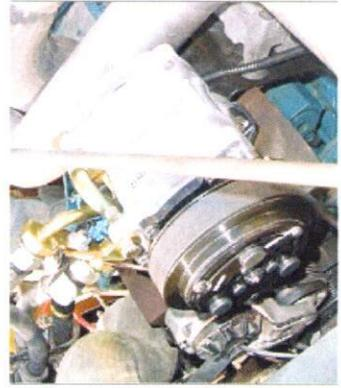
10. Position new compressor like removed compressor and secure with (Qty 4) 3/8" x 1" bolt. Torque to 28.9-32.9 ft-lb
